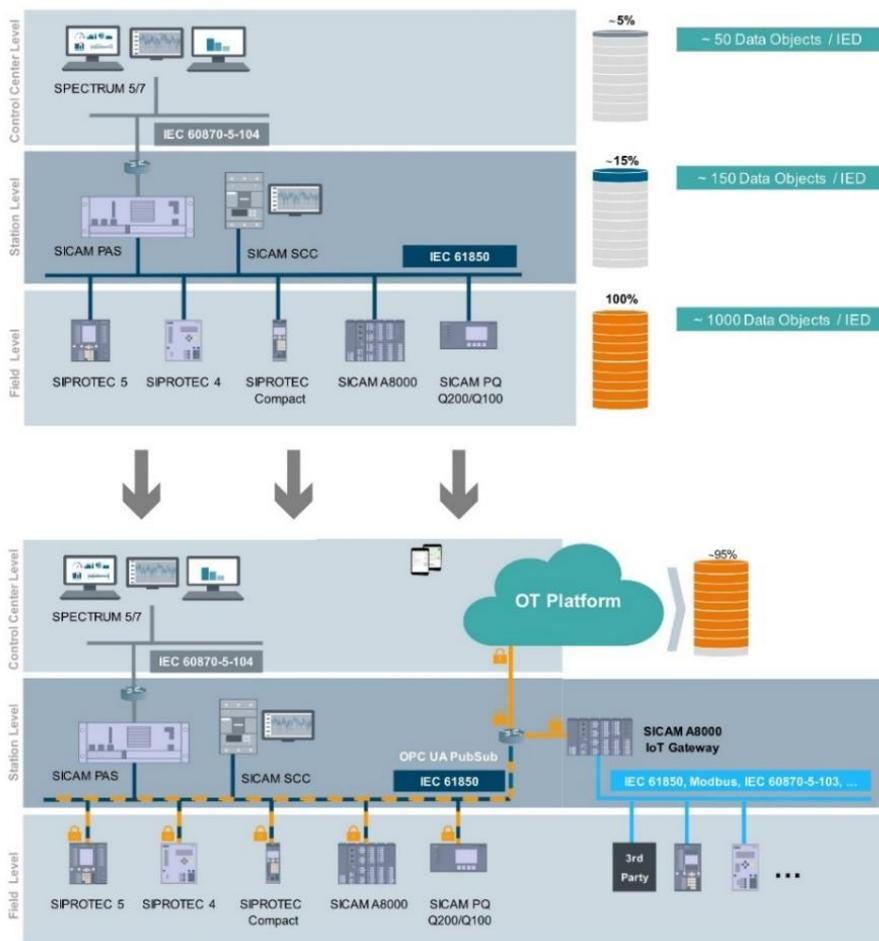
Image 1: Data Processing Layers in Power Grids
