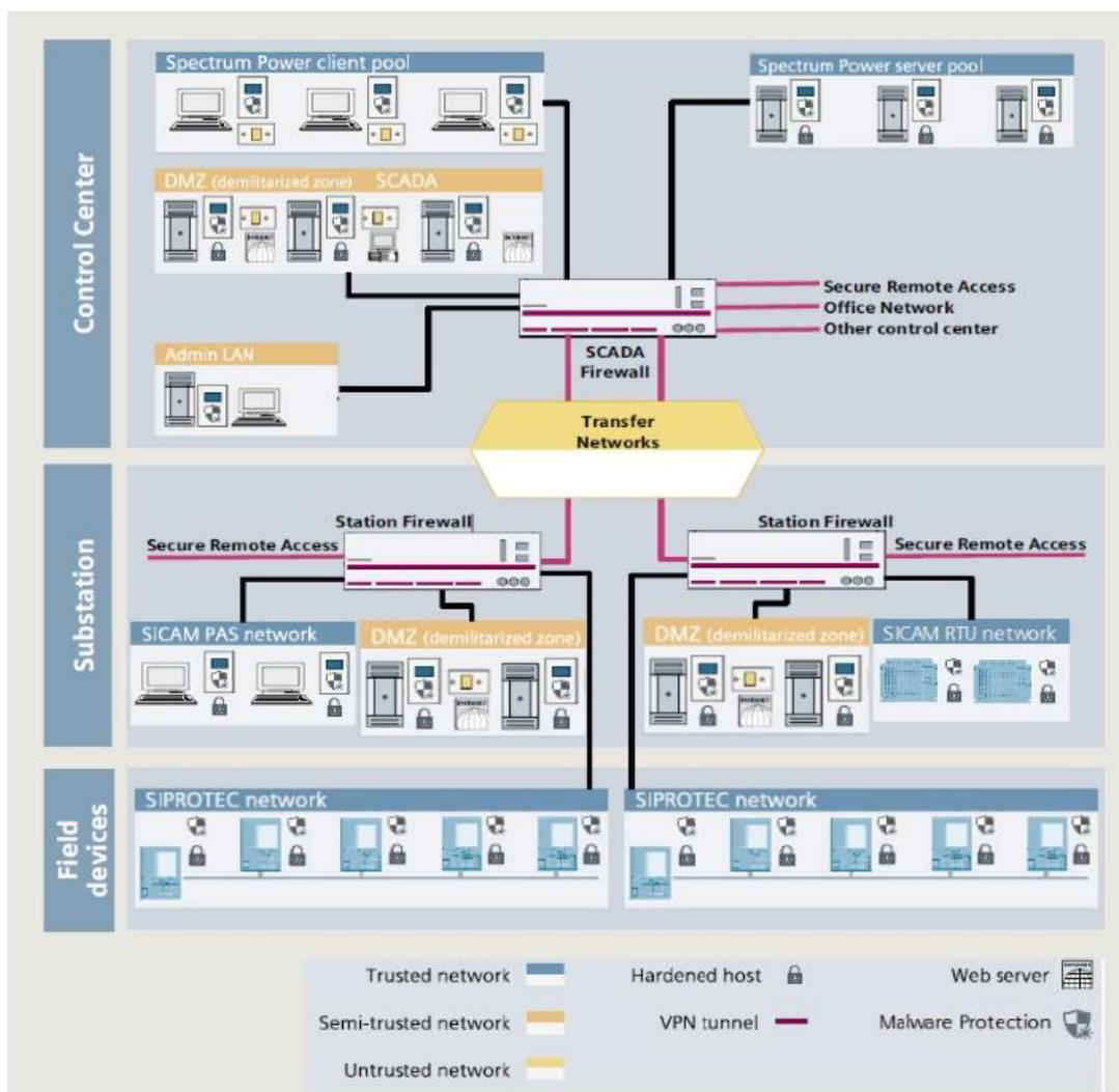
Image 7: Cyber Security Architecture for Power Grids
