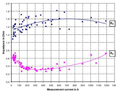
Figure 2: Measured zero-sequence impedance of a selected cable type
