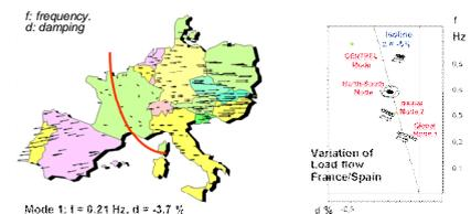
Figure 1: Inter-area oscillation after variation of load flow in France / Spain.
