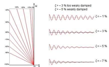
Figure 2: Criteria of weakly and well-damped system
