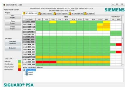
SIGUARD PSA protection performance visualization (color-code: red - fault not cleared, or orange/yellow - over-/ underfunction) In this state-of-the-art approach the protection system performance is as-
