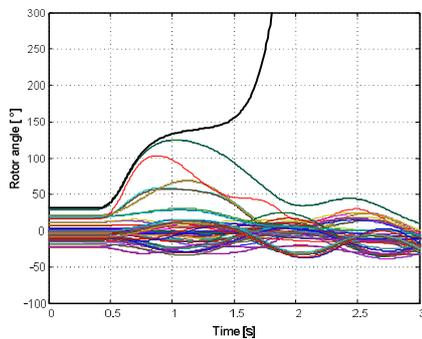
Figure 3: Transient stability after severe fault, a generator becomes unstable and is separated from the synchronous group
