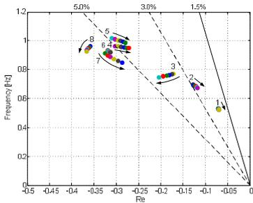
Figure 2: Presentation of system oscillation modes on complex plane with regard to variations in load or network topology alternations.
