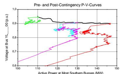
Figure 1: PV curves from four different working points, the red and magenta curves result in a voltage collapse.
