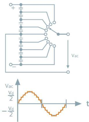
Figure 2: Basic HVDC Plus concept
