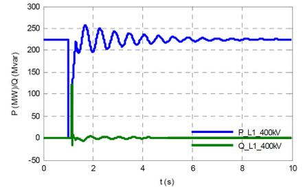
Figure 2: Real and reactive power curves during a fault-ride-through simulation
