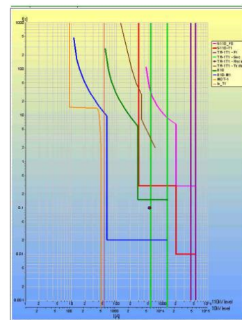
Figure 5: SIGRADE grading path and grading diagram
