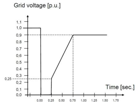
Figure 2: Example of a fault ride-through requirement curve
