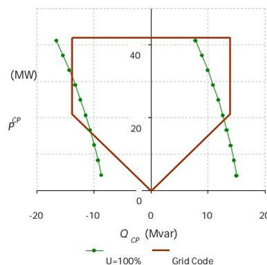
Figure 1: Example of reactive power capability curves
