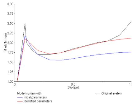
Figure 2: Results of a parameter identification of an induction machine
