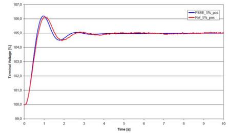
Figure 3: Graphical comparison of +5.0% voltage step change to AVR inertia (simulation and measurement)
