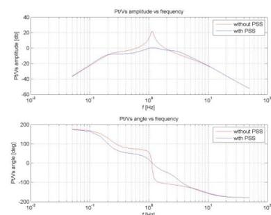
Figure 1: Bode plot with and without a power system stabilizer (PSS)
