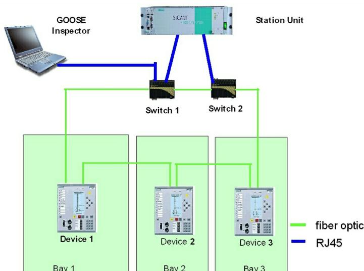
Figure 3: Schematic representation of the network structure
