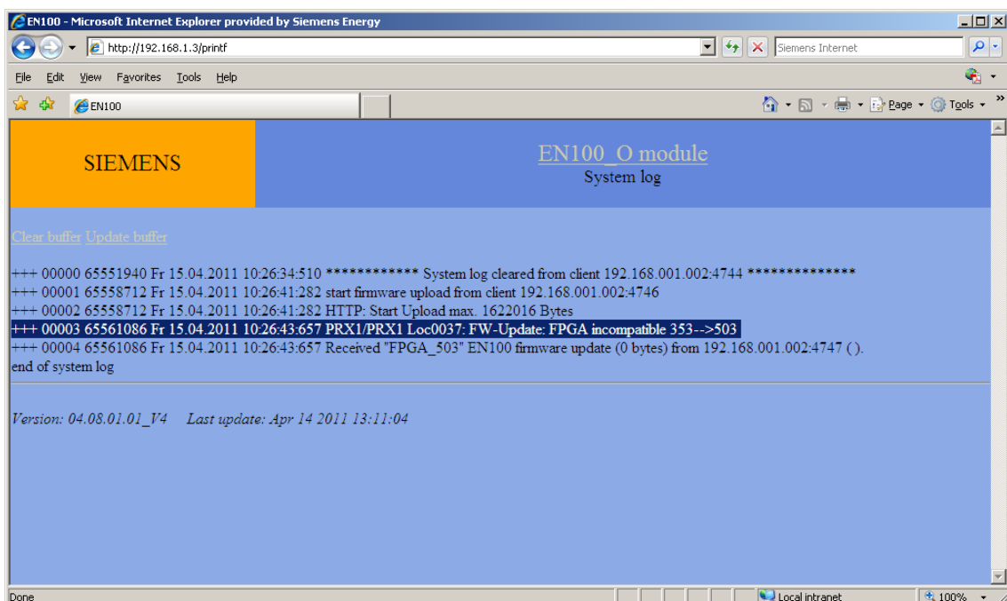
Figure 5-12 – System log after failed download – incompatible FPGA image for this hardware
