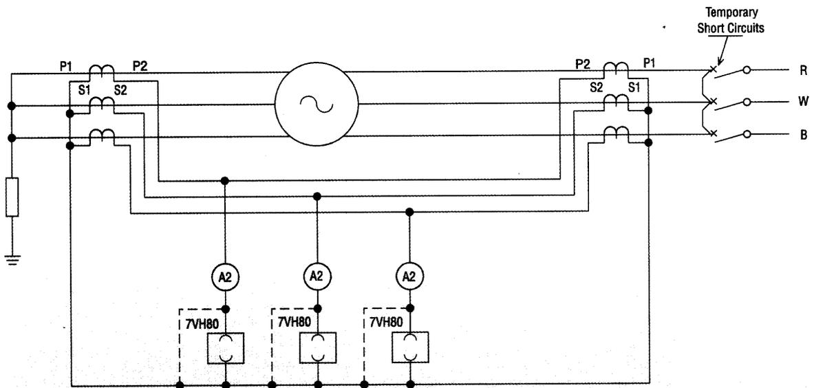
Fig 11. Through fault stability test
