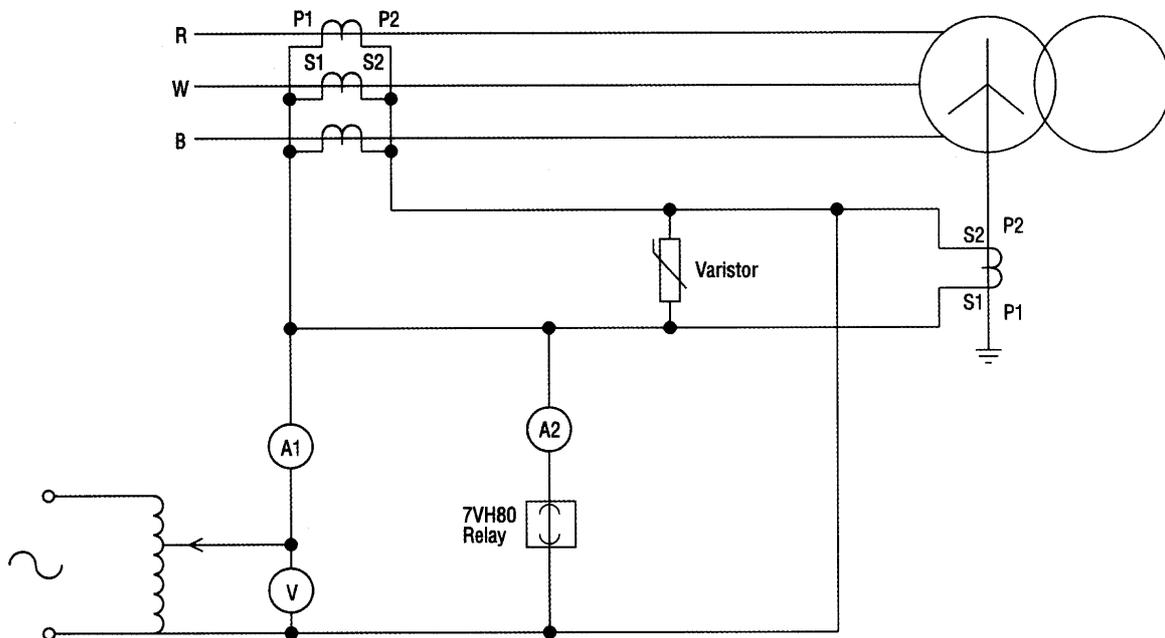
Fig 6. Secondary injection test
