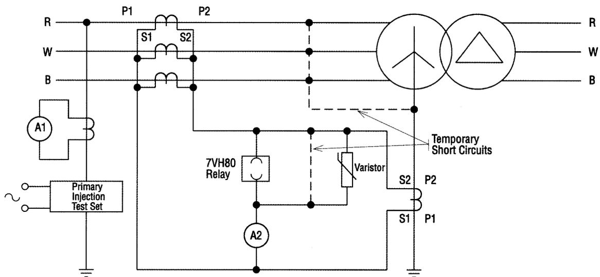
Fig 8. Through fault stability test
