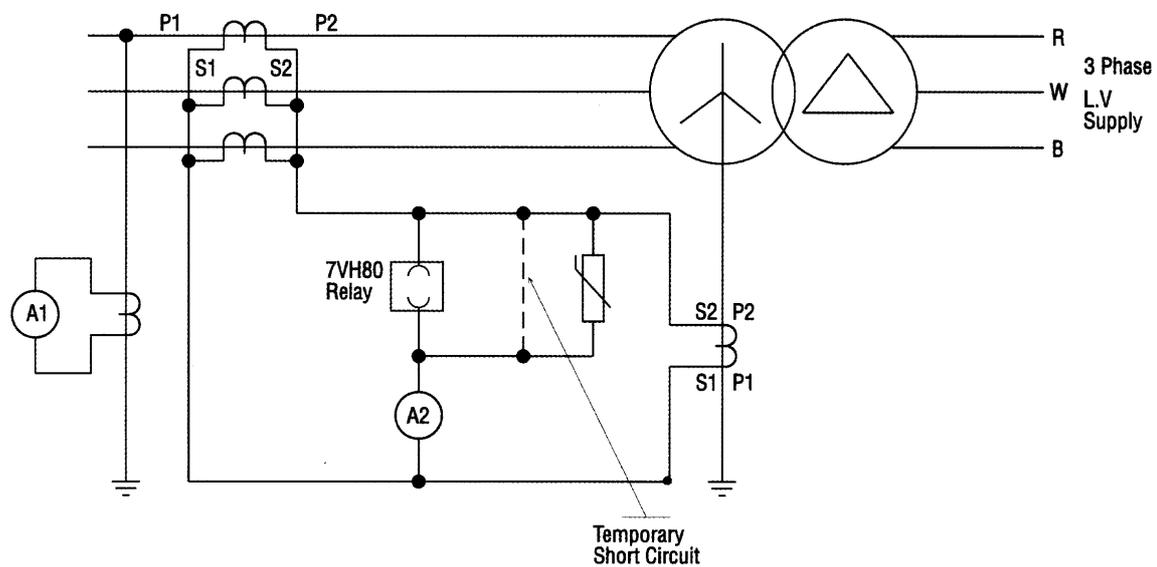
Fig 9. Through fault stability test
