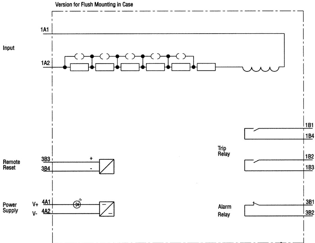
Fig 2. Connection diagram for 7VH80 relay
