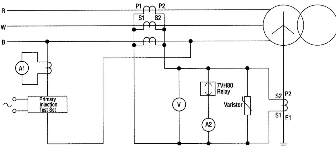
Fig 7. Primary fault setting test
