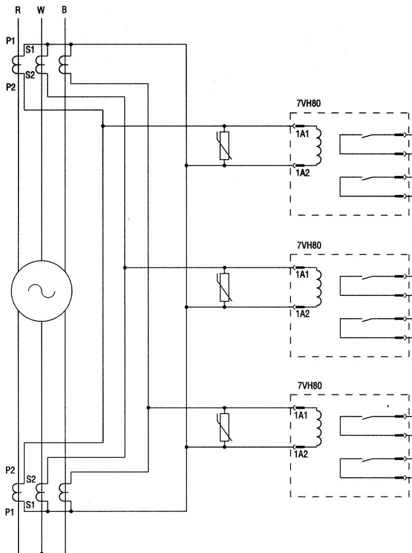
Fig 5. Phase and earth fault protection of a generator
