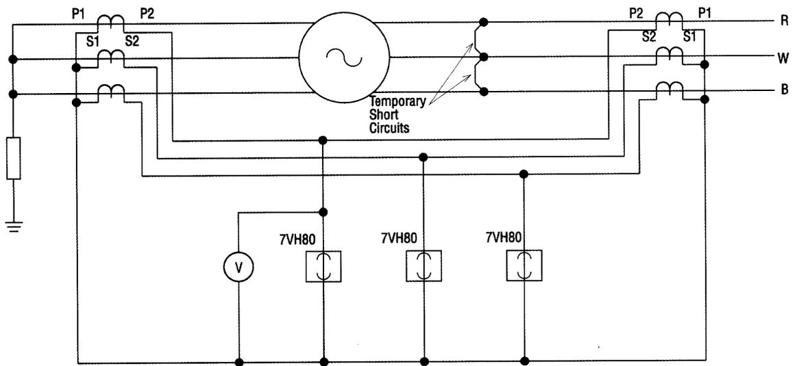
Fig 10. Primary fault setting test
