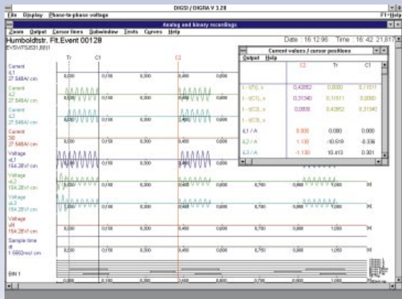
Fig. 5 Fault record of analog and binary traces
