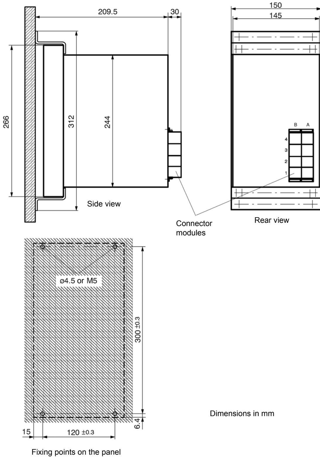
Figure 3 7XR61 Housing for panel surface mounting 7XP2030-1
