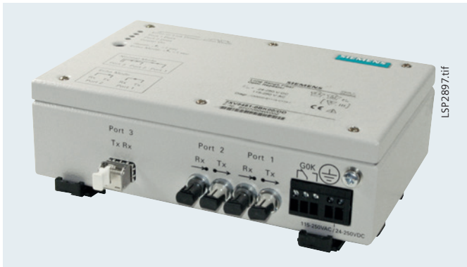
Fig. 13/44 Optical repeater with integrated 1300 nm/1550 nm wavelength multiplexer for one single mono-mode FO-cable
