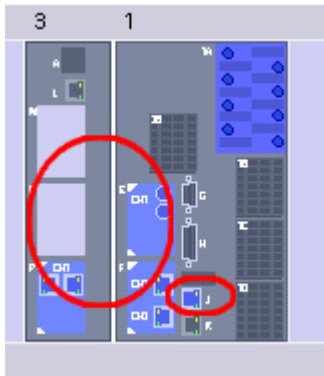
Figure 5-111 Inserting an Ethernet Module
