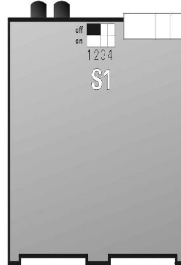
Fig. 3: DIP switches S1: 4 DIP switches
