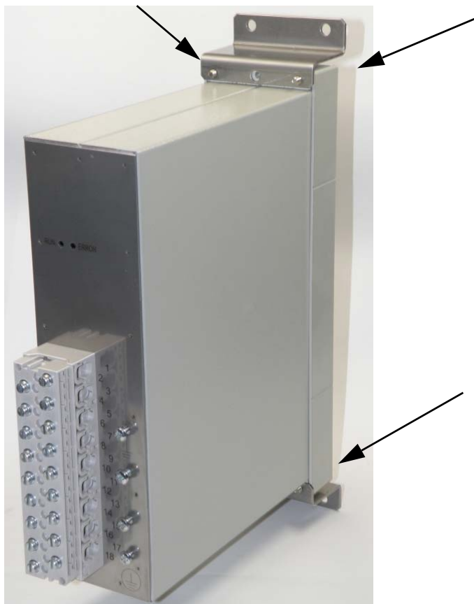
Fig. 8-2 Attaching the Z Angles to the Front Cover
