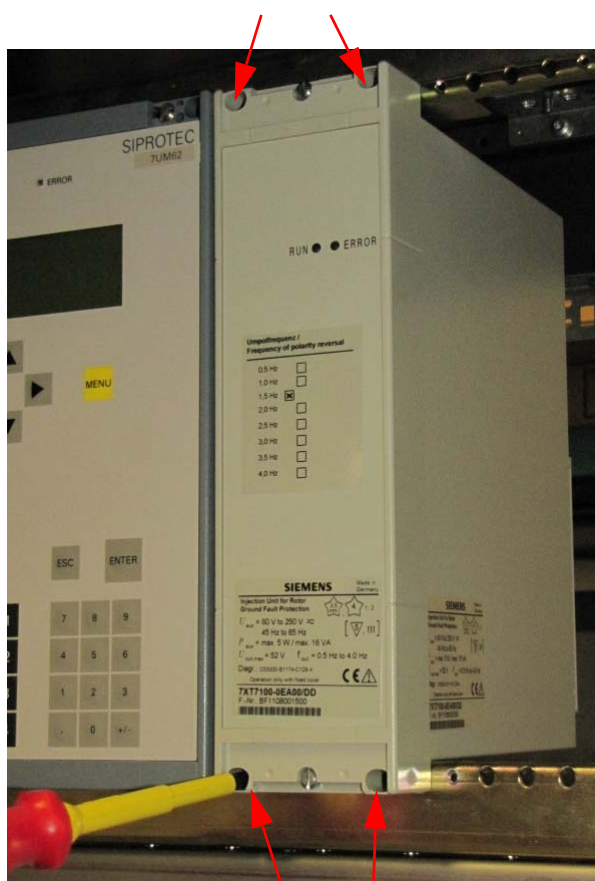
Fig. 8-3 Installing the Device into the Switch Panel
