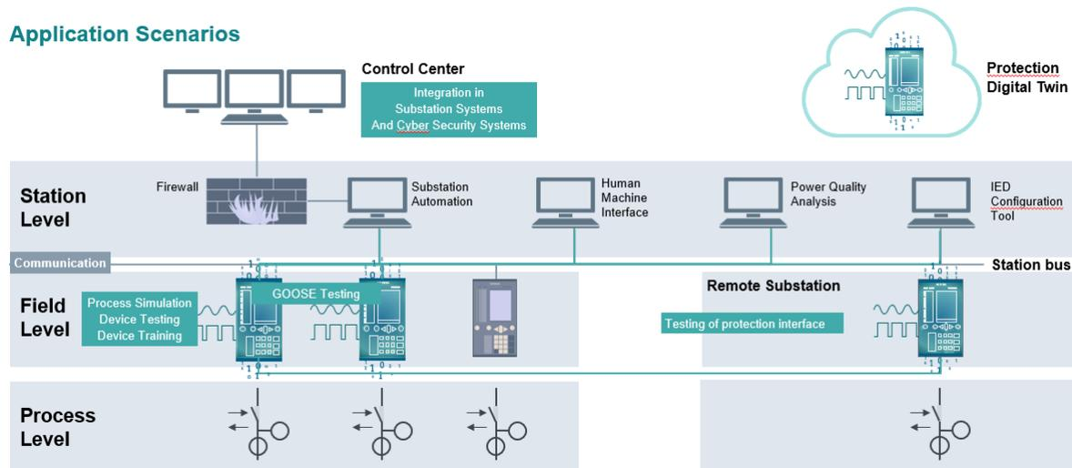
For the use of a protection digital twin, not only the IED behavior is required, but also the process simulation to provide the test inputs. This includes the virtual injection of both analog inputs such as currents and voltages, as well as of binary inputs. This process simulation may provide static inputs or more dynamic ones such as a COMTRADE replay.
