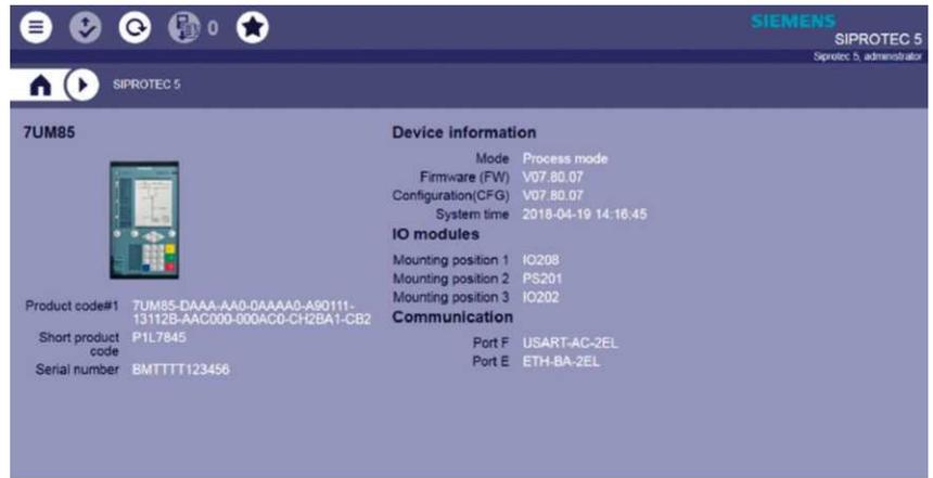
Figure 5. Web browser of Siprotec 5 - display of device data
