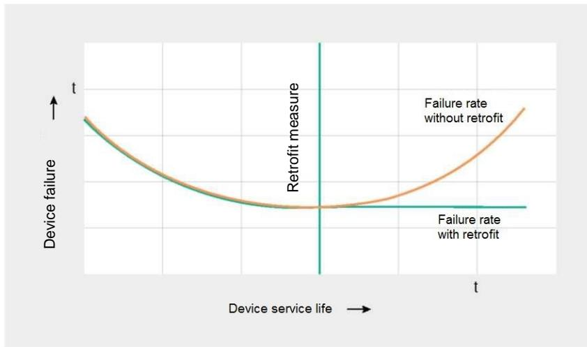
Figure 1. Graphic representation: Device failure in relation to device service life
