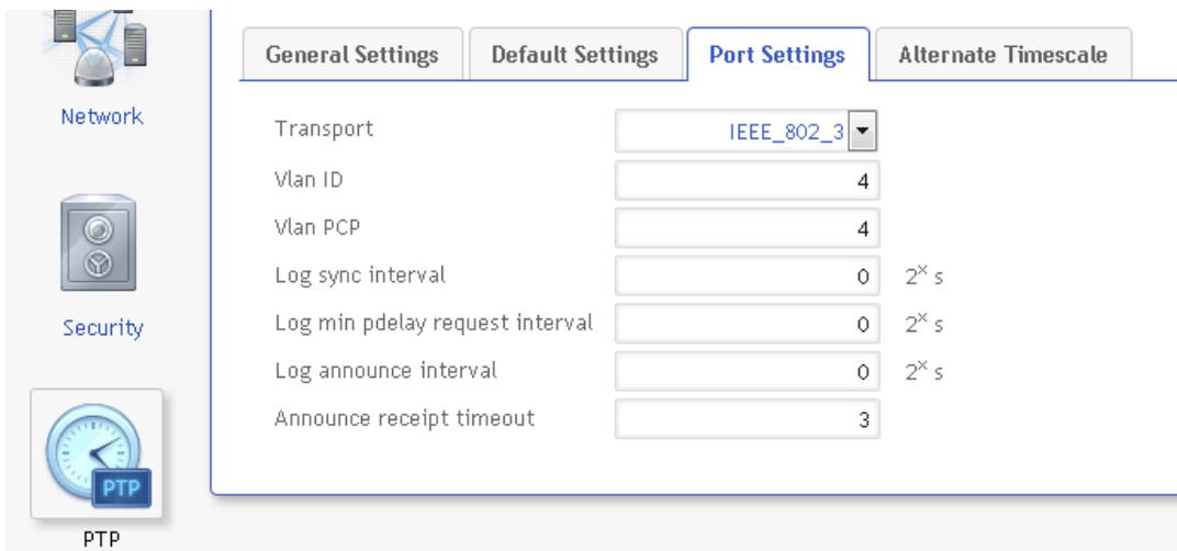
**Figure 10:** Settings of the VLAN ID of the OMICRON Lab OTMC 100p
