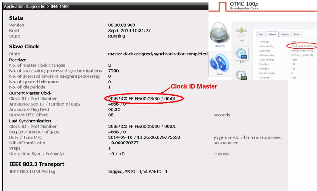
Figure 15: Homepage of the SIPROTEC 5 device and the web interface on OTMC 100p.
