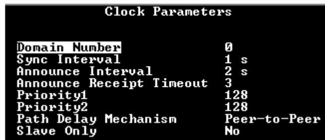
Figure 13: Console Clock Parameters
