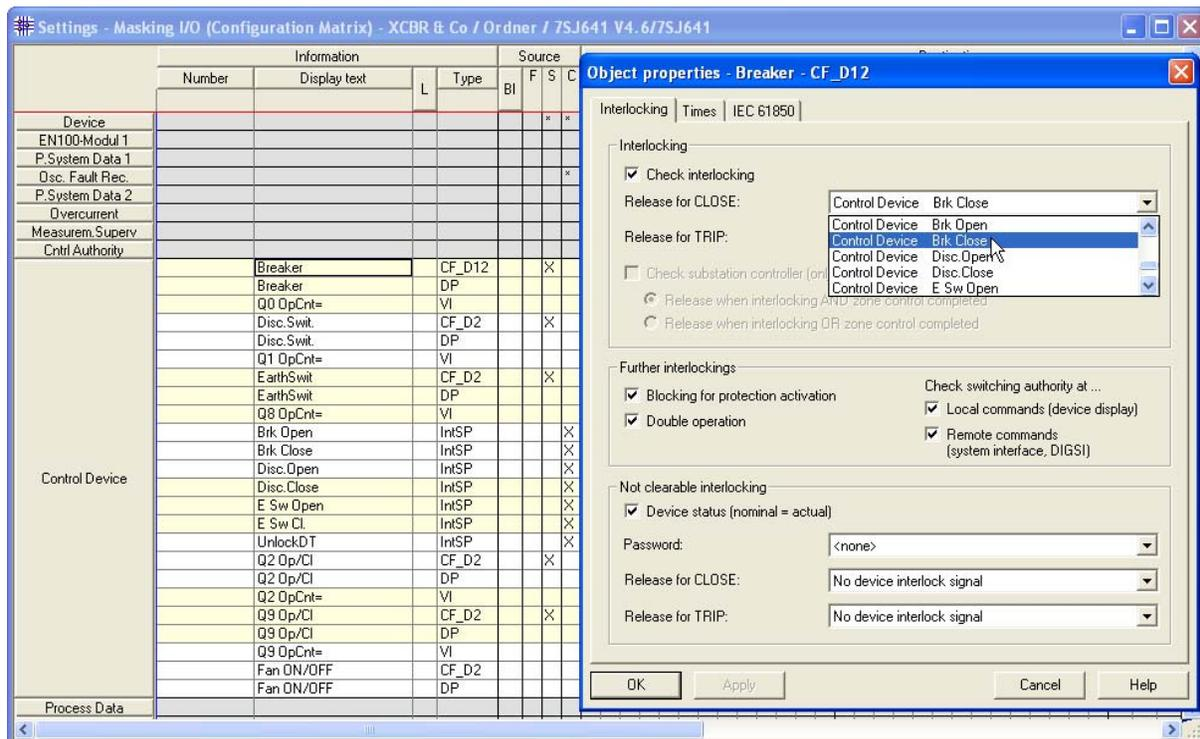
Picture 7: Object properties of the circuit breaker
