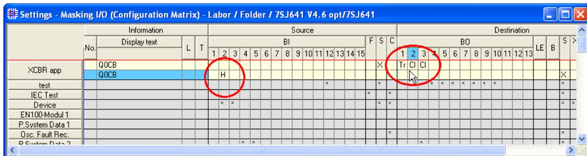
Picture 12: configuration of the source and destination of the circuit breaker
