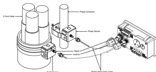
Figure 1-7 SICAM FPI connected with Phase and Earth Sensors
