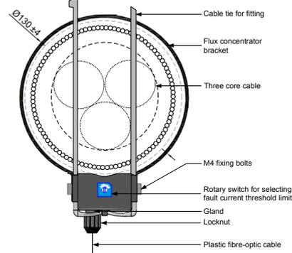
Figure 1-8 Earth Sensor Installation
