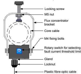
Figure 1-6 Phase Sensors Installation
