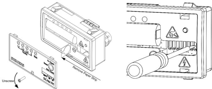
Figure 1-3 Removal of Paper Strip and DIP Switch Settings
