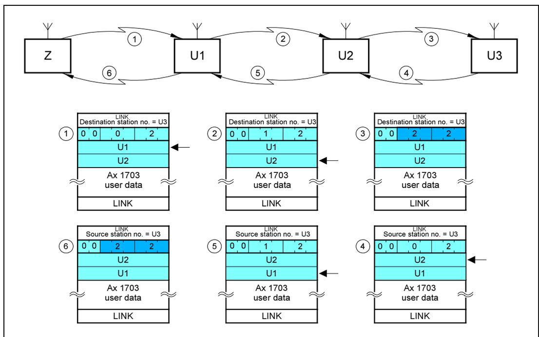
Example of the management of the routing information for 2 intermediate stations (routing stations)
