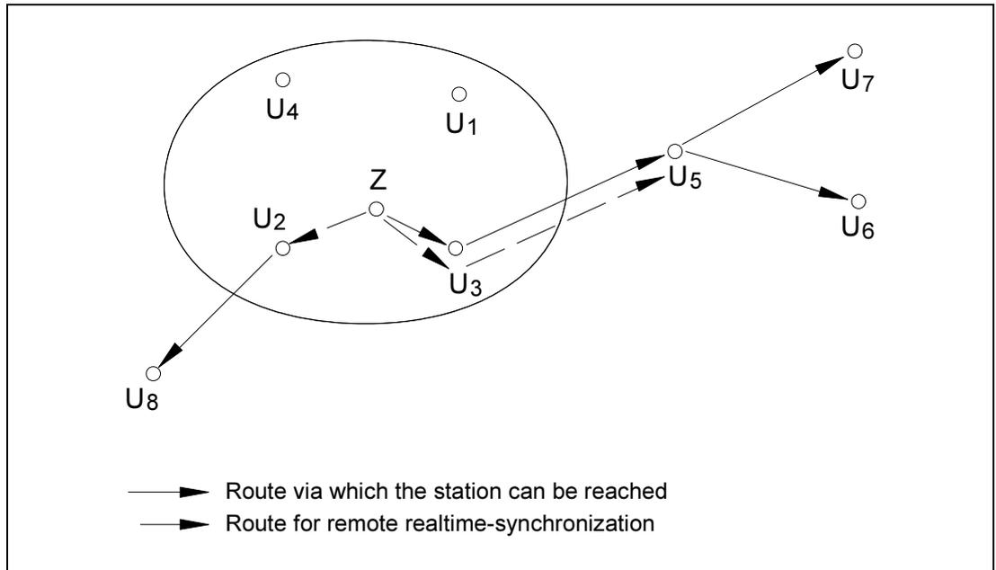
In this special case, a time synchronization is sent to stations  $U_6$  and  $U_8$ . Stations  $U_6$  and  $U_7$  can be reached via  $U_3$  and  $U_5$ .
