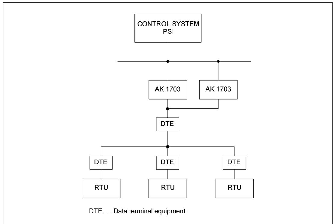
Every RTU is issued with a component number based on the station number (St#). Each station must also be issued with a region number via the topology parameterization (all stations of a line must have the same region number).
