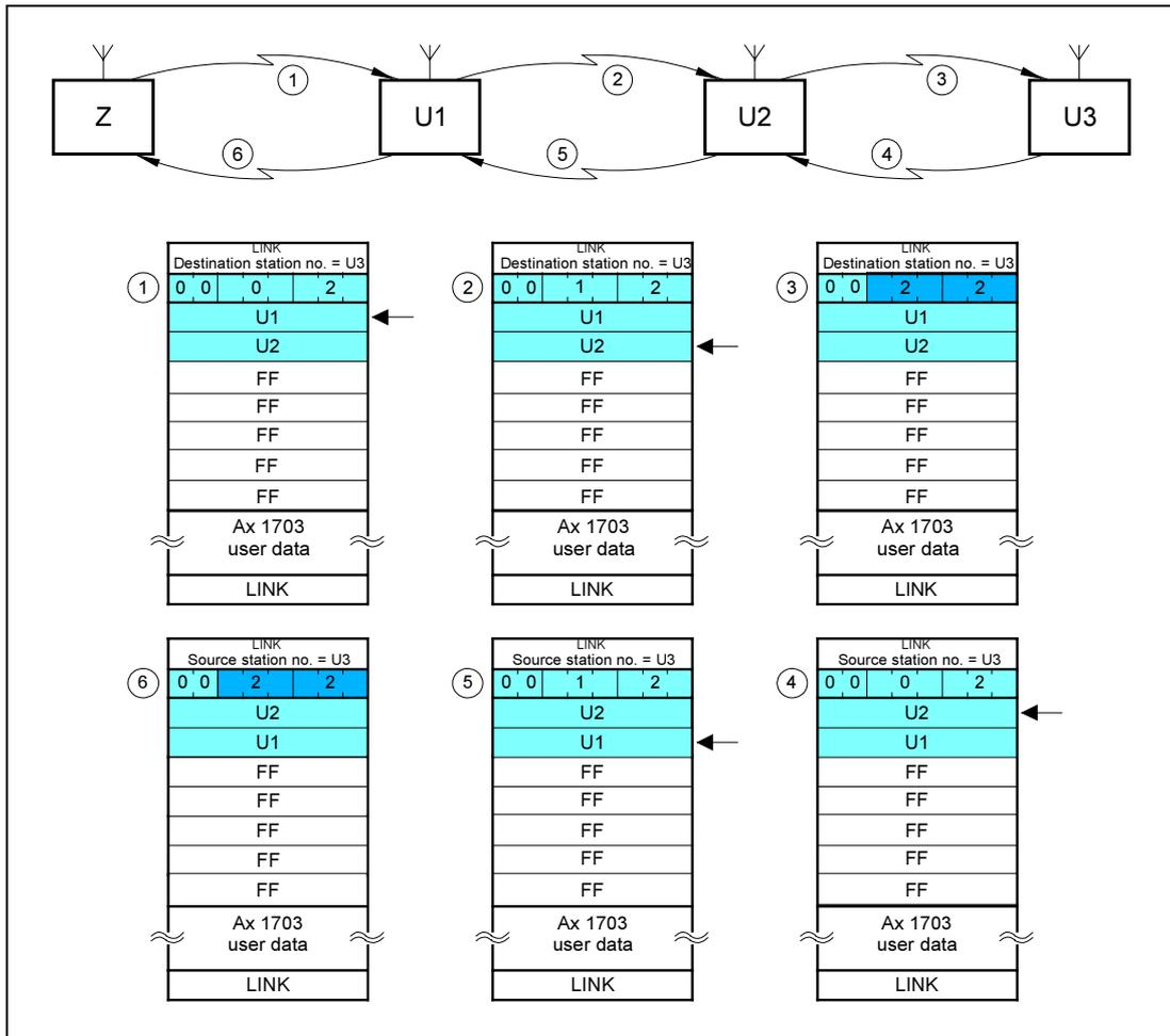
*Example of the management of the routing information for 2 intermediate stations (routing stations)
