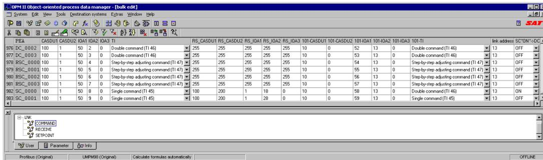
Example for "SIP message address conversion" for UMPM98 in control direction for single-double commands
