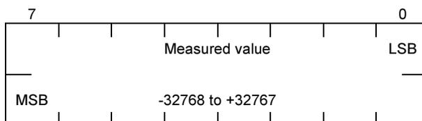
*Object format DNP V3.00 16 Bit Frozen Analog Input with Time of Freeze:*
