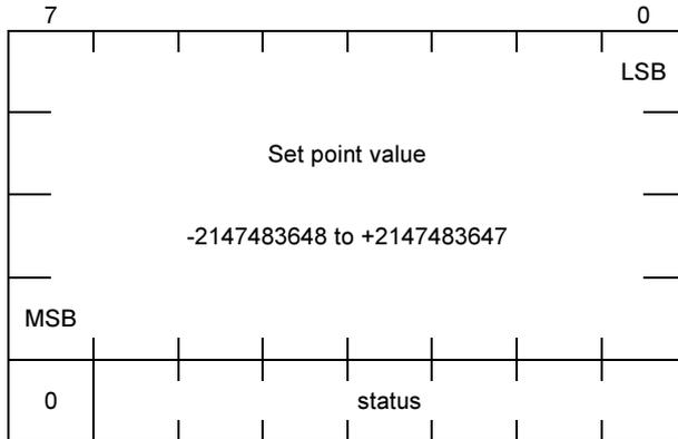
*Object format DNP V3.00 16 Bit Analog Output Block:*
