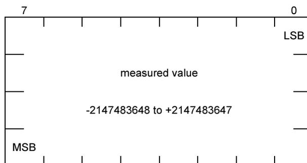
*Object format DNP V3.00 32 Bit Frozen Analog Input with Time of Freeze:*
