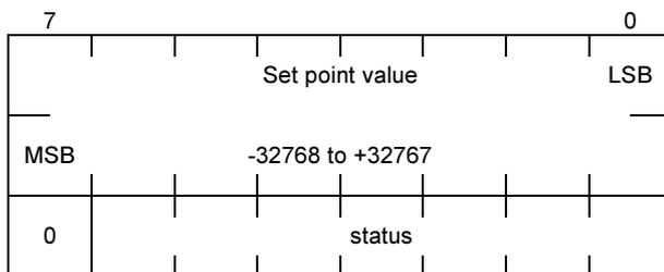
*Object format DNP V3.00 Short Floating Point Analog Output Block:*
