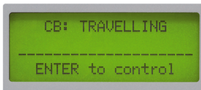
Fig.4 Example of Control Function View
