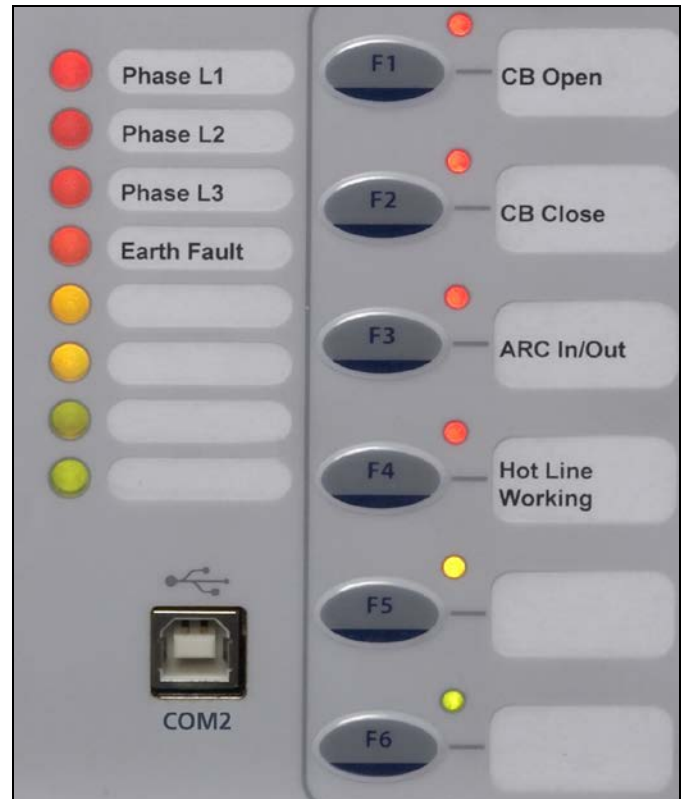
Fig 1. Tri-colour LED's and function keys
