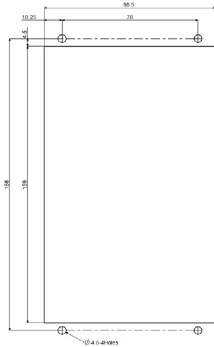
Fig 16. Panel cut-out View
