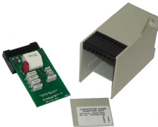
Fig 3. Capacitor Cone Adaptor Unit construction
