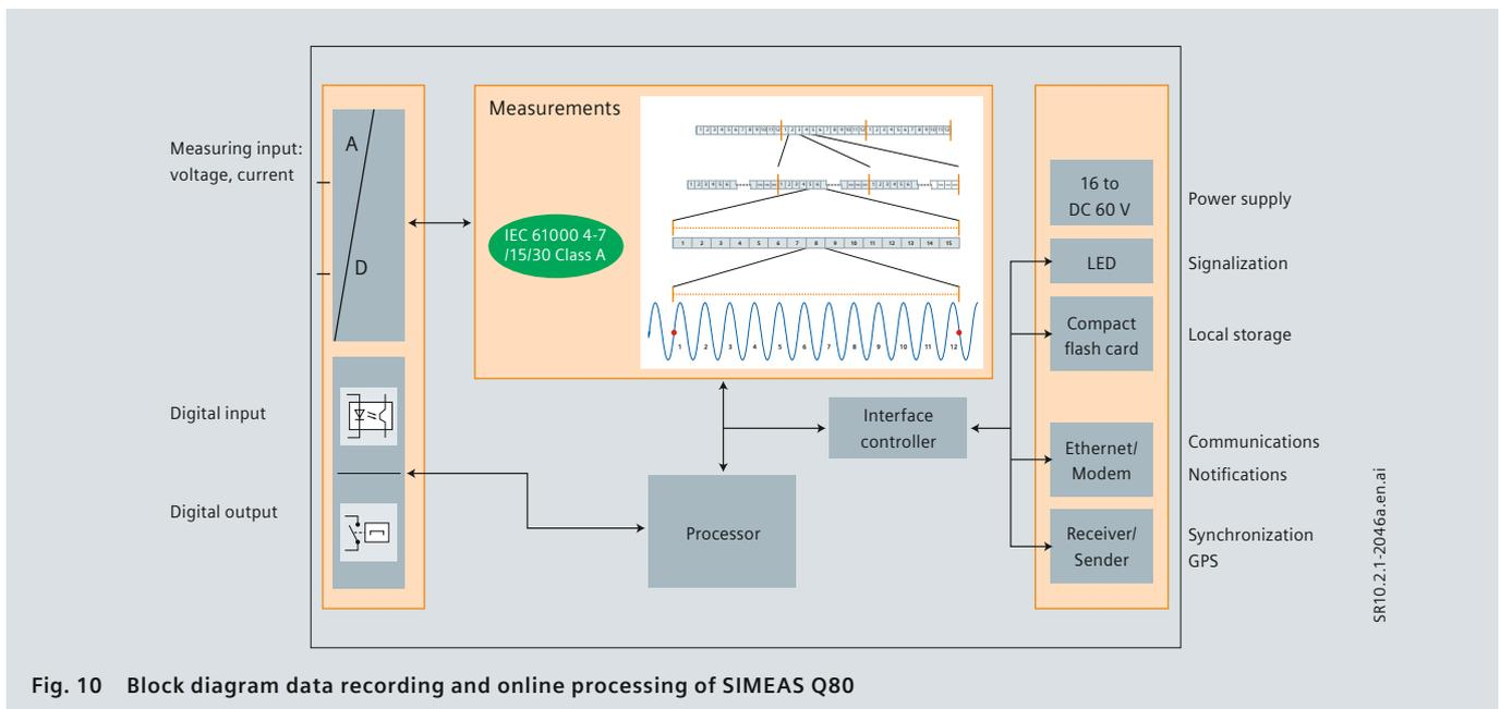
Fig. 10 Block diagram data recording and online processing of SIMEAS Q80
