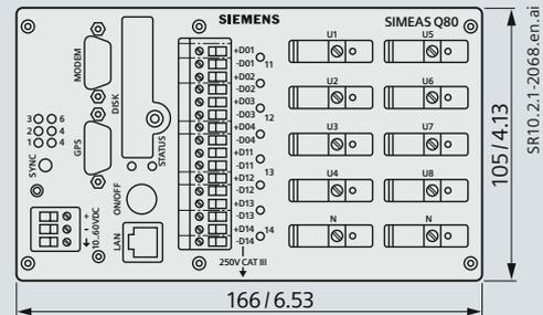
Fig. 32 7KG8080 – eight-voltage connection: front view
