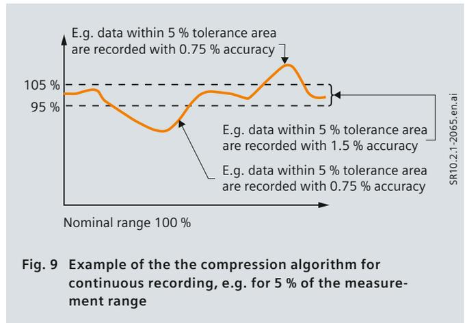
Fig. 9 Example of the the compression algorithm for continuous recording, e.g. for 5% of the measurement range
