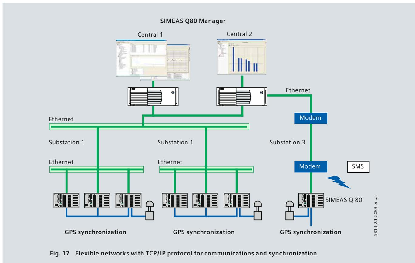
Fig. 17 Flexible networks with TCP/IP protocol for communications and synchronization
