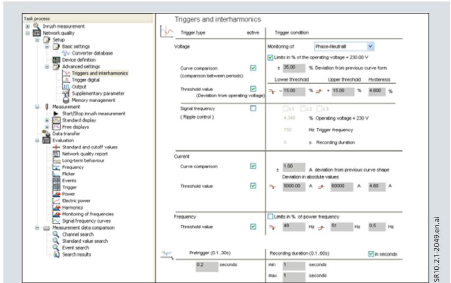
Fig. 13 Trigger parameterization
