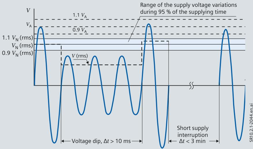
**Fig. 6** Illustration of a voltage dip and a short supply interruption, classified according to EN 50160;  $V_N$  – nominal voltage of the supply system (rms),  $V_A$  – amplitude of the supply voltage,  $V(rms)$  – the actual rms value of the supply voltage
