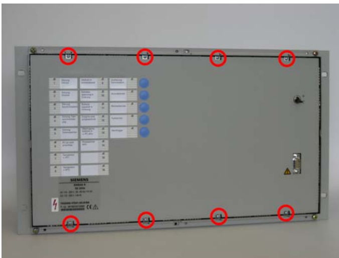
Figure 39: Removing the front panel
