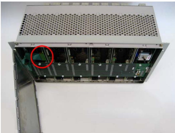
Figure 41: Connection of ribbon cable
