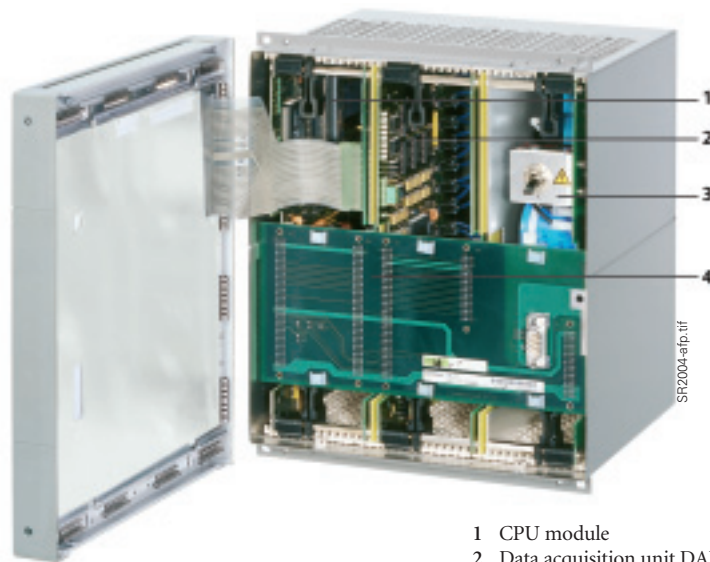
Fig. 13/71 Layout of a SIMEAS R
