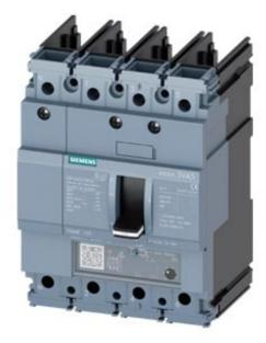
circuit breaker 3VA5 UL frame 125 breaking capacity class H 65kA @ 480V 4-pole, line protection TM230, FTAM, In=100A overload protection Ir=100A fixed short-circuit protection Ii=5...10 x In N conductor protection 100% without connection
