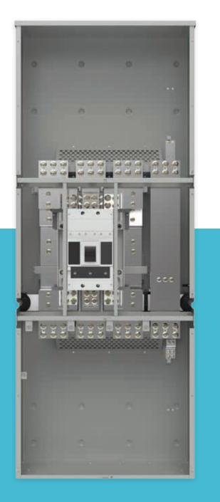
Imagine a four-story building designed with a group metering line up on each floor. If the total load is between 1,200 and 2,000 amps, one BFT module can be placed on the first floor as the main for the first floor's meters and the service entrance main for the entire building using feed-through tapboxes on the second and third floors and a standard breaker main or WTB tapbox on the fourth floor.
