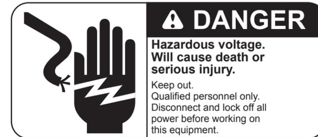
1. Lock off all power supplying this equipment before working on it.
