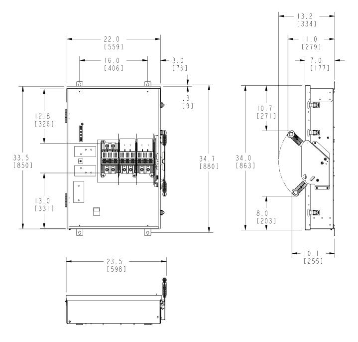
Dimensions shown in inches and millimeters [ ]. Dimensions shown accurate to  $\pm$  1/8 inch.
