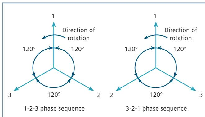
The phasor diagram represents the phasor (or vector) relation of the three phase-ground voltages (for simplicity, in a balanced system). The diagram is based on counter-clockwise rotation, and in a system with 1-2-3 phase sequence, the voltage with respect to time in phase 1 reaches a peak, followed 120 electrical degrees later by phase 2, and similarly, phase 2 is followed 120 electrical degrees later by phase 3.
