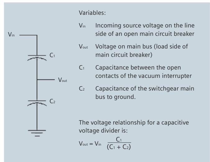
In this example, when energized at 13.8 kV phase-phase (8 kV phase-ground), the expected voltage on the load side of the main circuit breaker (in this example, on the main bus) with all feeder and tie circuit breakers open would be:
