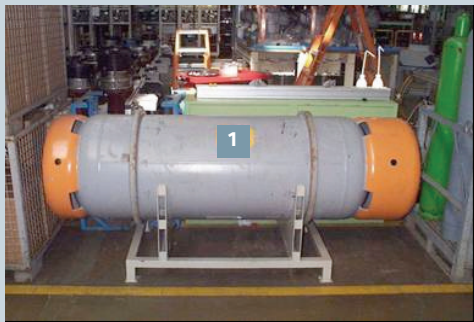
1. Cylinder for storage of gas to be recycled
