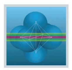
The SF<sub>6</sub> molecule, has six fluorine atoms placed symmetrically around a sulfur atom. The symmetrical arrangement leads to extreme stability, a very desirable characteristic for an insulating gas. This gives the gas a very high dielectric capability, approximately three times the dielectric strength of air at atmospheric pressure. As a result, equipment using SF<sub>6</sub> as an insulating medium can be considerably more compact than equipment using air as the insulating medium.
