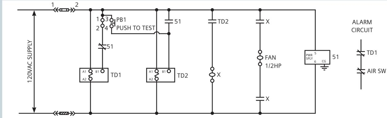
Typical fan-cooling control circuit schematic diagram
