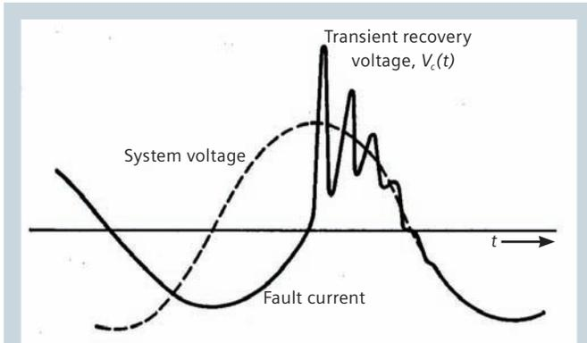
Figure 2: TRV vs. system voltage and current
