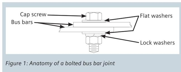
Figure 1: Anatomy of a bolted bus bar joint
