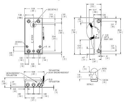
Dimensions shown in inches and millimeters (). Dimensions shown accurate to  $\pm \frac{1}{l_8}$  inch
