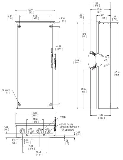
No knockouts in enclosure. Dimensions shown in inches and millimeters ( ). Dimension shown accurate to  $\pm\,\%$  inch.
