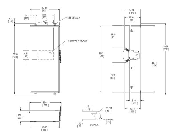
No knockouts in enclosures. Dimensions shown in inches and millimeters ( ). Dimension shown accurate to  $\pm\,1\!\!/\!_{2}$  inch.
